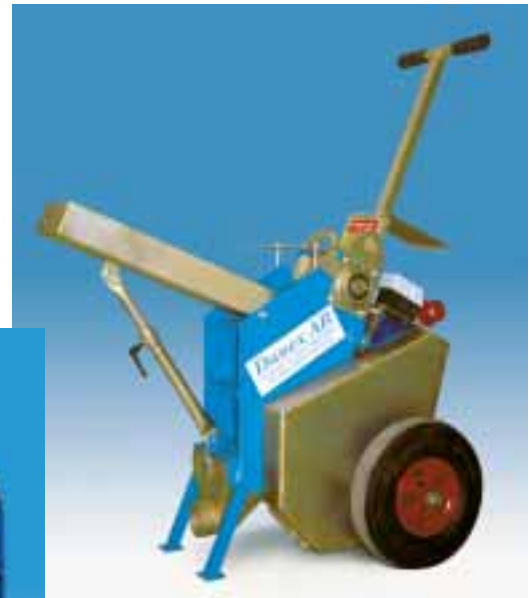
DX 3 Intended for fragmentation and removal of demolition material, especially when renovating bathrooms.
